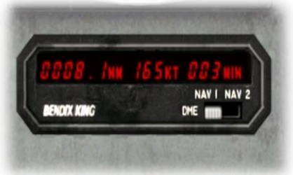
Distance Measuring Equipment (DME) Master Display
