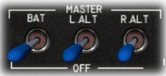
Master Electrical Switches
