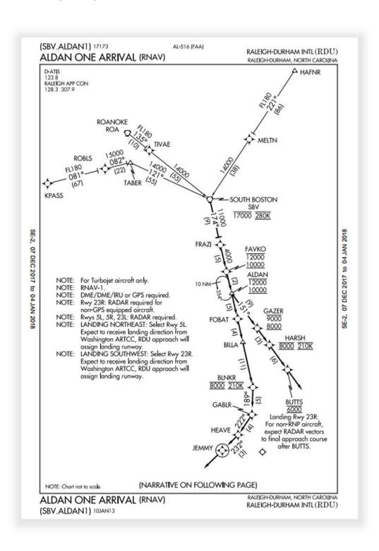
The ALDEN ONE procedure is for turbojet aircraft equipped with RNAV1 capability only. RNAV1 capability means that the aircraft can maintain a total system error of not more than 1 nautical mile for 95% of the total flight time.
