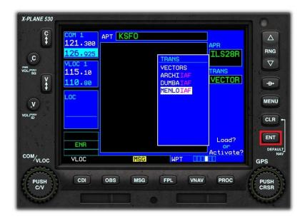
Click the GPS Inner Rotary at the 3 O'clock and 9 O'clock positions to select the desired initial approach fix (IAF). You may select VECTORS in place of an IAF, if ATC is providing these.
