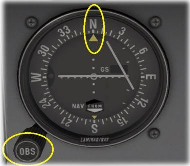
• Select the desired bearing, which, in this example, is 360 degrees
