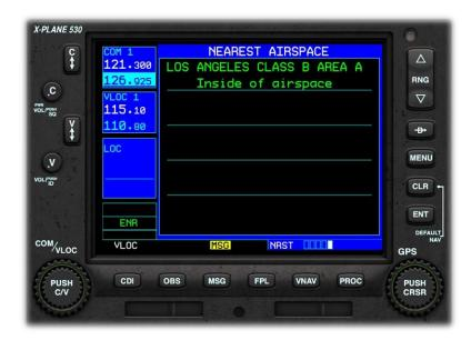
This Page displays the nearest controlled, or special-use, airspace to your current location, together with the airspace type.
