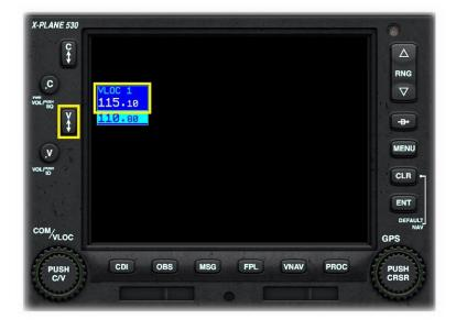
Click the VLOC (VOR / Localizer) Frequency Flip-Flop Key to swap the standby and active NAV frequency.
