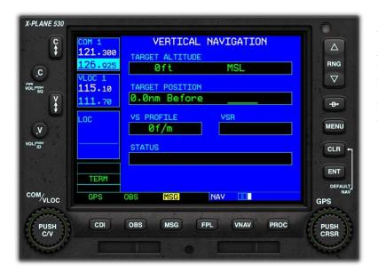
The Vertical Navigation (VNAV) Page provides the capability to designate a target altitude for a <u>single</u> waypoint in your flight plan. This feature is only active during the execution of a flight plan, or a "Direct To" instruction. As you approach the designated waypoint, the VSR and STATUS data fields on the VNAV Page will provide guidance to ensure the target altitude is achieved.
