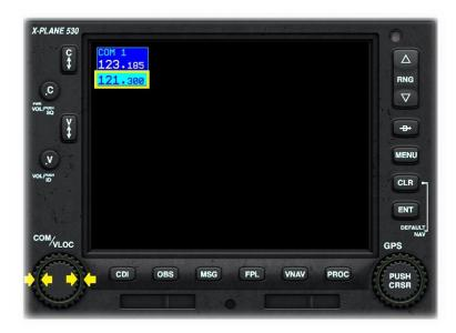
Click the CENTER of the Comm / VOR Localizer Rotary to highlight the standby COM frequency.
