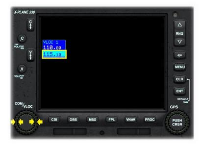
Click the CENTER of the Comm / VOR Localizer Rotary to highlight the standby NAV frequency.
