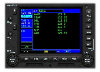
This Page displays the frequencies associated with the destination airport, (or current airport where no destination is specified).
