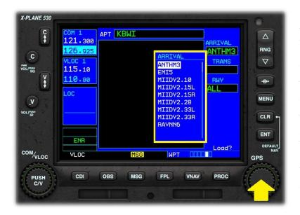
This Page displays supports the selection of the desired STAR (Standard Arrival) procedure for the destination airport.
