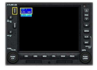
Click the Comm Frequency Flip-Flop Key to swap the standby and active COM frequency.
