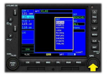
This Page displays supports the selection of the desired SID (Standard Instrument Departure) procedure for the airport of origin.
