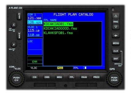
This Page displays the catalog of saved flight plans that currently exists in the following folder:
